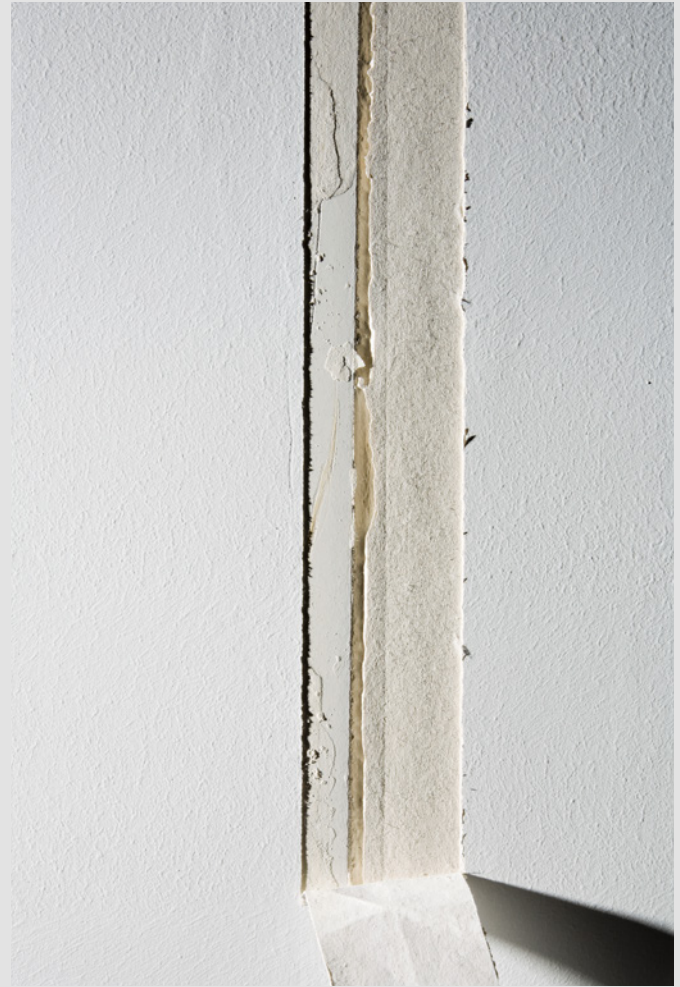
Cause: Too little jointing compound under the joint tape on the cut edge side (left of the joint centre)
