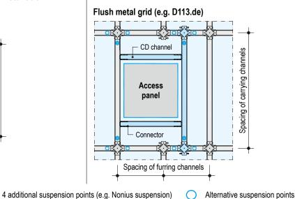
Universal connectors are required for the trimmers. Further suspenders are required if the suspended profiles are to be exchanged.
