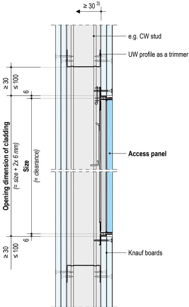
3) Opening displacement clearance of the access panel
