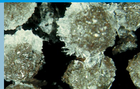
Salt capillary structure under the microscope
