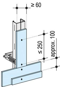
Board offset 1st layer to 2nd layer Diamant approx. 100 mm
