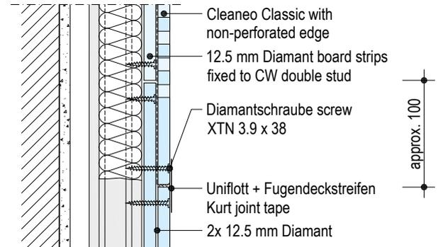
W629C.de-VU20 Floor connection to basic floor slab
