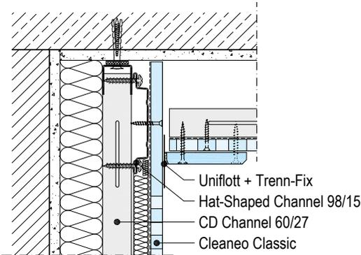
W623D.de-VM1 Board joint on Hat-Shaped Channel
