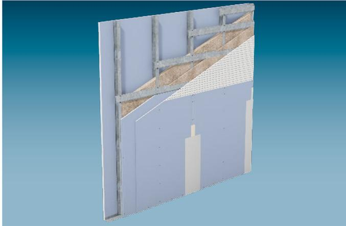
The Cleaneo Acoustic Wall **W112C.de** is an absorber partition implemented as a hybrid construction that meets the sound insulation requirements while improving the acoustic quality of the room thanks to its sound absorbing properties.
