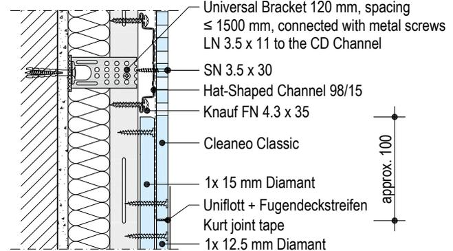
W623D.de-VU2 Floor connection to basic floor slab
