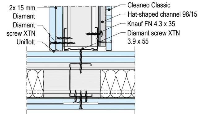
With wall height > 3.00 m and demands on the fire resistance, backing of the CW perimeter connection profile on the web side is required.
