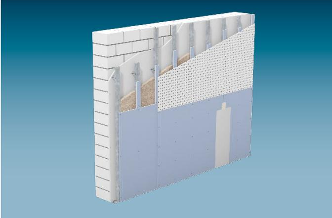
The Cleaneo Acoustic Wall Lining with board strips **W623C.de** is implemented with a grid made of sheet metal profiles CD 60/27, that are fixed to the basic wall with Universal Brackets. Thus a slim construction method is assured. The cladding in the Cleaneo Classic area is backed on the studs with additional Diamant board strips. In the non-perforated area two layers of Diamant GKFI 12.5 are to be applied.
