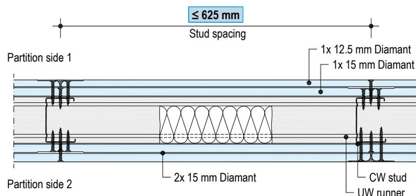
W112C.de-B2 Board joint, non-perforated area
