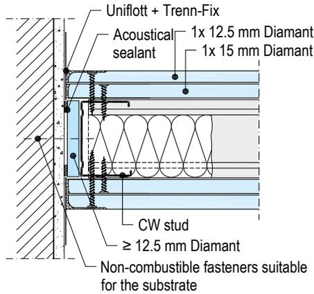
With wall height > 3.00 m and demands on the fire resistance, backing of the CW perimeter connection profile on the web side is required.
