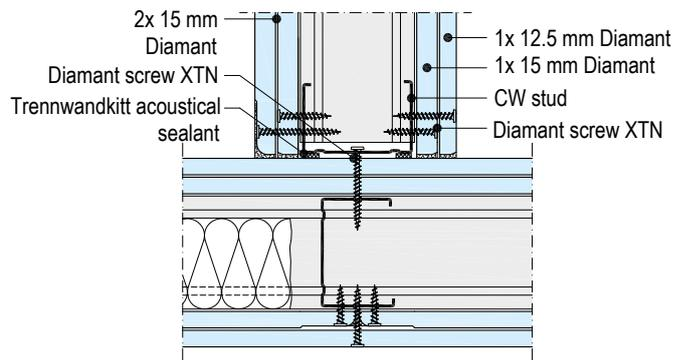
With wall height > 3.00 m and demands on the fire resistance, backing of the CW perimeter connection profile on the web side is required.
