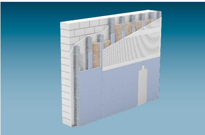
The Cleaneo Acoustic Furring **W629C.de** is implemented with a grid made of CW sheet metal studs as a double stud frame as a free-detached arrangement in front of the basic wall. Due to the free-detached arrangement there is no dependence on the strength of the basic wall. The cladding in the Cleaneo Classic area is backed on the studs with additional Diamant board strips. In the non-perforated area two layers of Diamant GKFI 12.5 are to be applied.
