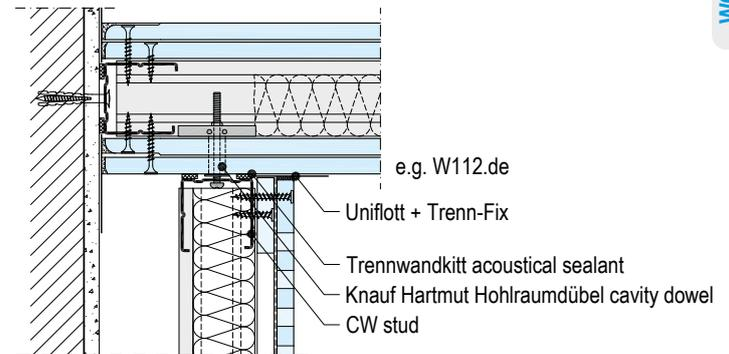
**W112C.de Construction design, ball impact safe**
