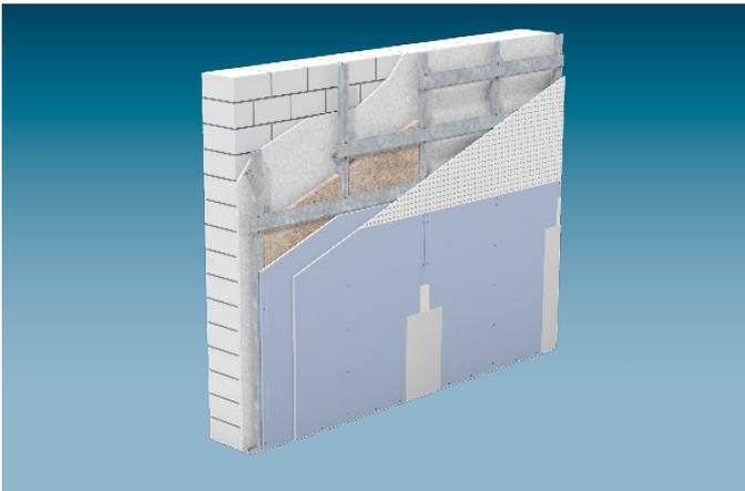
The Cleaneo Acoustic Wall Lining with Hat-Shaped Channel **W623D.de** is implemented with a grid made of sheet metal profiles CD 60/27, that are fixed to the basic wall with Universal Brackets. Thus a slim construction method is assured. The cladding in the Cleaneo Classic area is backed with additional Hat-shaped channels. In the non-perforated area two cladding layers of Diamant GKFI (15 + 12.5) to be applied.
