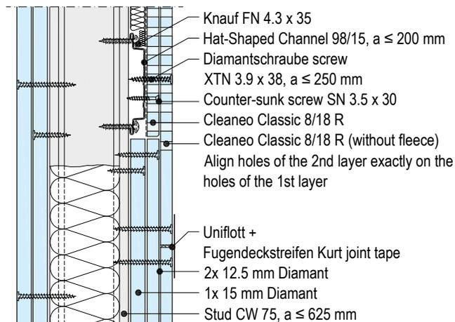
**W623C.de Construction design, ball impact safe**
