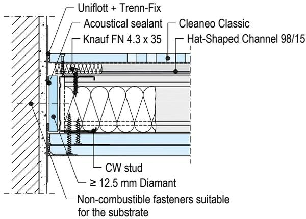
With wall height > 3.00 m and demands on the fire resistance, backing of the CW perimeter connection profile on the web side is required.
