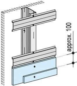
Board offset 1st layer to 2nd layer Diamant approx. 100 mm
