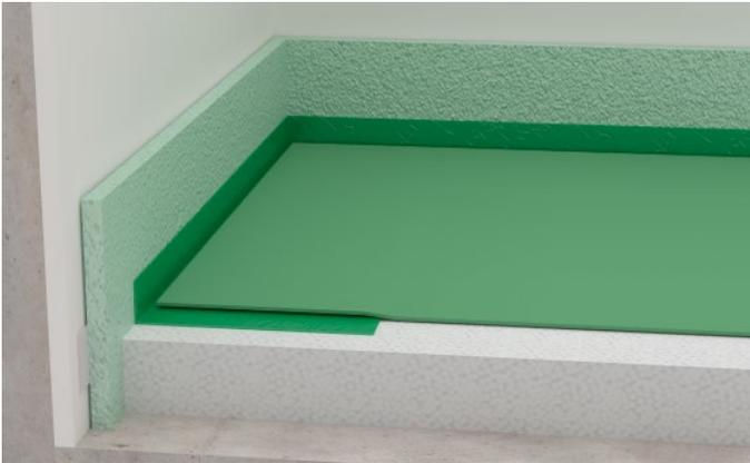
3. Lay Schrenzlage synthetic coated kraft paper with an overlap of at least 80 mm on the joints. On the connection to the walls, they are applied to the installed foil strips of the edge insulation strip.
