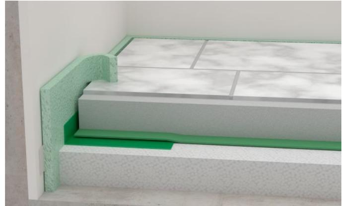
5. Only remove the protruding part of the edge insulation strip (in acc. with DIN 18560-2) after the floor covering is applied.
