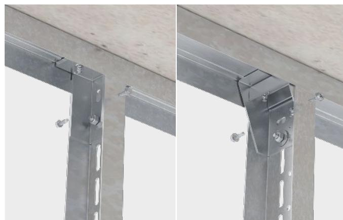
Screw fasten the UA profile using the 2 enclosed bolt screws onto the side of the support base side wall or angle bracket flange. Subsequently tighten the M8 screws.
