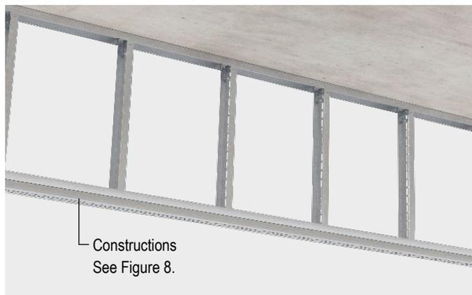
Push on the UW runner construction, fix and ensure correct alignment.
