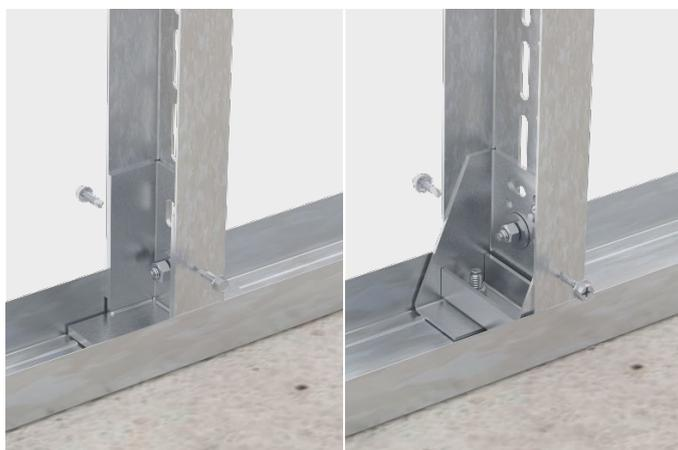
Screw fasten the UA profile using the 2 enclosed bolt screws onto the side of the support base side wall or angle bracket flange. Subsequently tighten the M8 screws.
