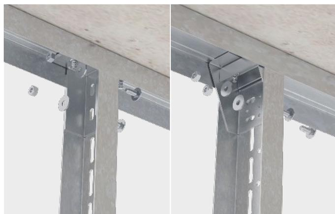
Cut the UA profile to the required length. Plug it onto the support base or angle bracket and screw it hand tight using the enclosed M8 screws with washers and nuts. Adjustability of the profiles for alignment purposes is required.
