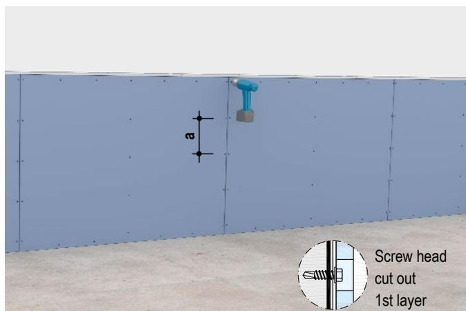
Cladding on both sides as well as on the top side with 12.5 mm Diamant boards.
